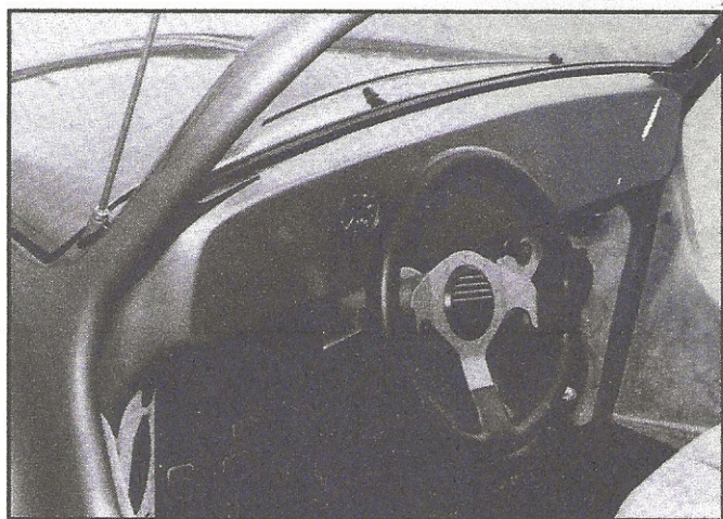
Not one area of the interior was left untouched! Even the dash was smoothed-out displaying only a VDO speedo, two emergency lights and a Formula France steering wheel.
