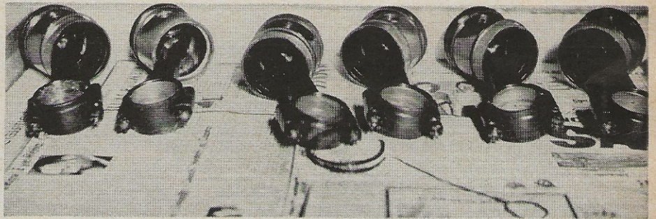
Number-two piston's short skirt and missing bottom ring reveal makeshift repair.
