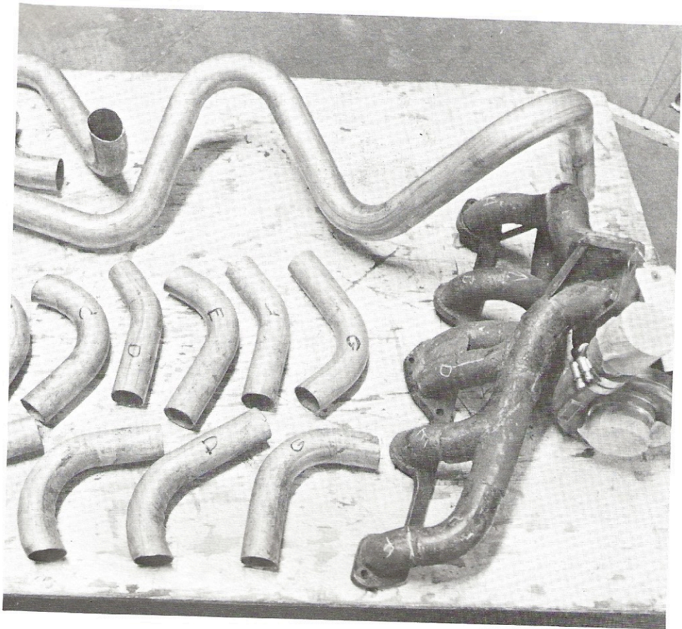
JIGSAW PUZZLE???—This is a prototype exhaust header, made from stainless steel to withstand the higher operating temperatures required with turbocharging. Ed Mills photos
