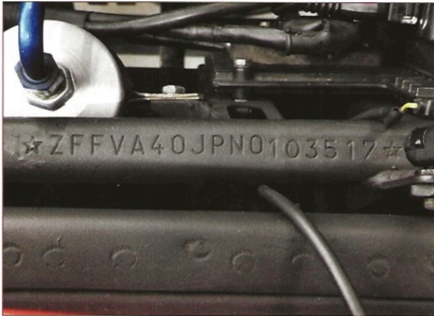
Foto punzonatura telaio (sul telaio) Photograph of the chassis number (on the chassis)
