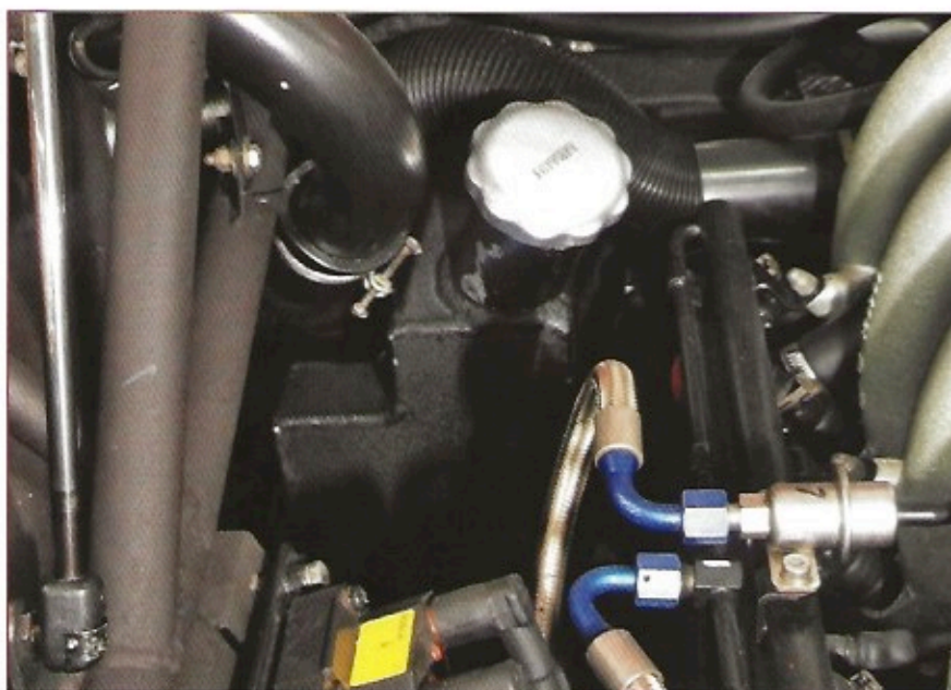
Serbatoio olio Oil tank
