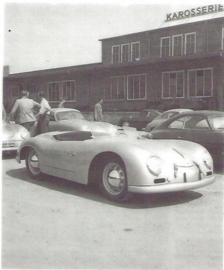
The Sauter Porsche from 1951, based on a 356 body. Most important, visible changes: doors for the Sauter Porsche were hinged at the rear and a cover could be bolted over the rear seats.
