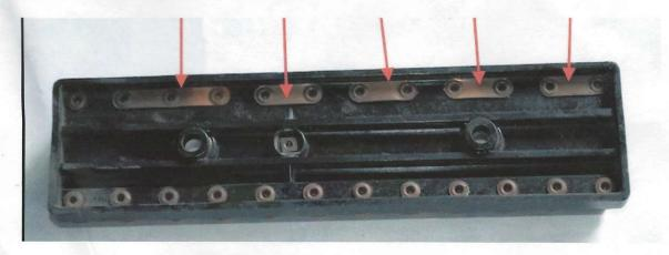
Install the ReFuze panel using the provided 4mm screws. 12 position panels have symmetrical mounting holes, take care to orient the ReFuze panel the same as the OEM block using the underside label as a guide.
