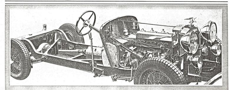
The Cruciform Braced Chassis Frame
