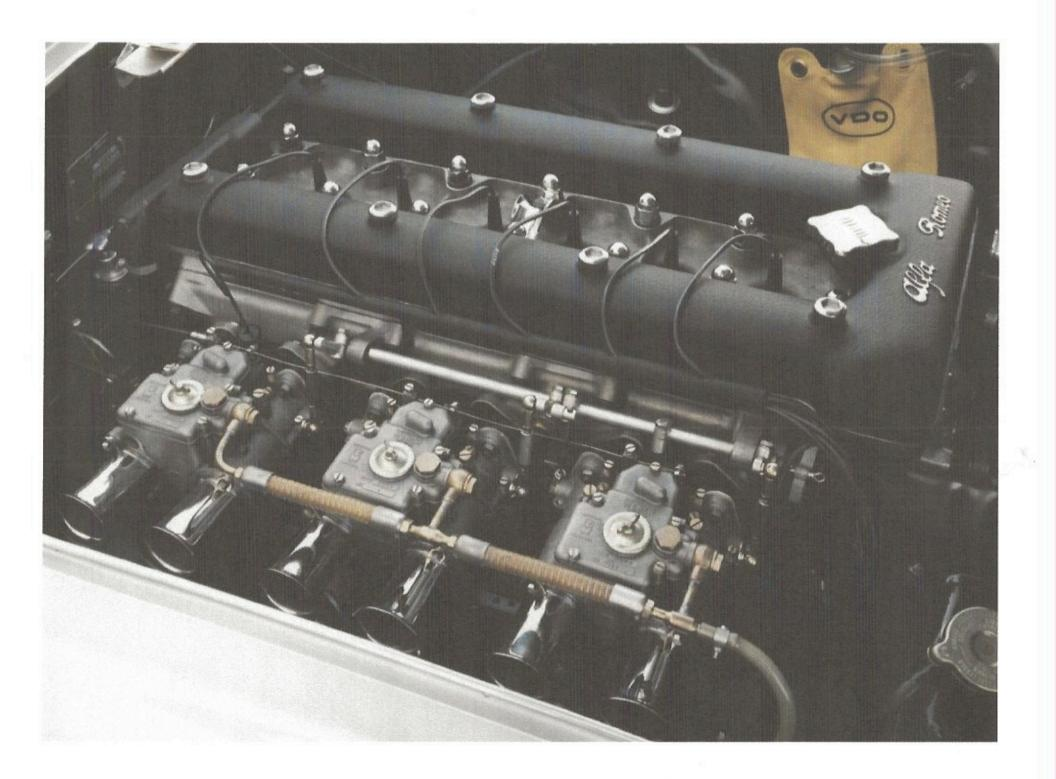
Laurence Anderson of Berkeley, CA restored all of this car's mechanical and electrical systems. The engine was completely torn down and all wearing parts replaced before being blue printed and reassembled. The induction, exhaust, cooling, oil, brake and electrical systems were similarly restored. Without Mr. Anderson's wealth of experience with vintage Alfa's, a complete and historically accurate restoration of this 2600 Spider would not have been possible.
