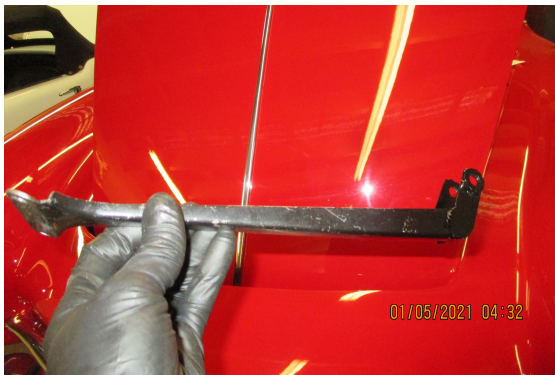
Remade carb support bracket to clear carb linkage, new spark plug wire set.
