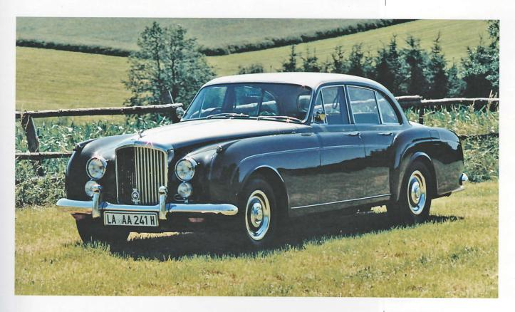
Flying Spur Design no. 7508 for the S 2 Continental was the evolution of that already seen on the first Series, but with the new Continental frontal styling with the lower radiator grill inclined forward. The other change was at the rear, with the deeper boot lid that incorporated the rear number plate. The last cars were equipped with new rear lamps that would be seen on the third Series.
