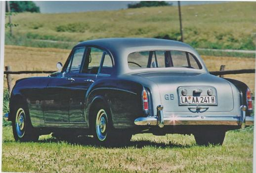
At the rear, the boot lid now incorporated the registration plate, improving the access to the boot floor. (20)
