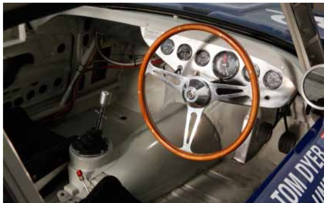
Clockwise, from main: model’s often-tricky handling has been refined on this racer; stripped-out cabin; 15in wheels allow bigger brakes; oil cooler
