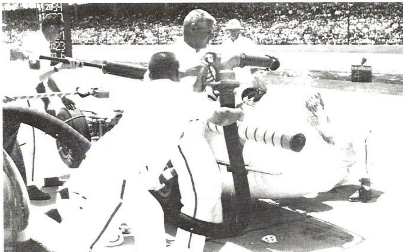
The hose valve fails to shut off completely and highly inflammable fuel is spilled in Rodger Ward's pit; luckily no fire resulted.
