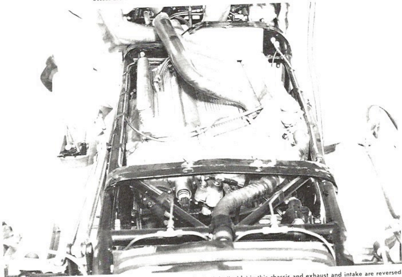
Offy is mounted rigidly in frame of conventional car at firewall and at removable front support. Simplicity of installation and easy access are criteria. Vibration is something builder has to live with.
