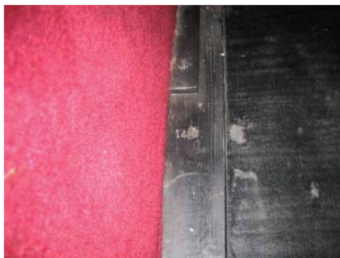
(Above) Vanden Plas body number 1486, stamped into the longitudinal runner to the rear floorboard (left) and the bottom timber to the nearside in front of and to the left of the front passenger seat (right). These numbers were stamped to ensure that floorboards, seats, windscreens, etc went back to the correct bodyshell after going through detail shops at Vanden Plas' works at Kingsbury.
