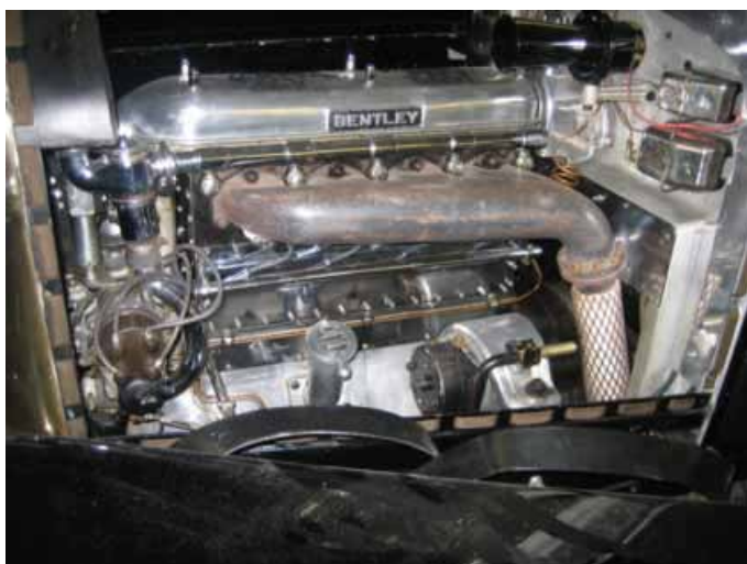
(Left) Nearside of the engine compartment, showing, correct for a 1928 4½ Litre, ML magnetos (either ER4 or GR4), thermostat housing, Smiths starter motor, round flange exhaust manifold, Smiths cut-out and fuse box to the front face of the bulkhead. (Right) Nearside engine bearer showing the original engine number TX3241 and the original pattern clip for the starting handle.
