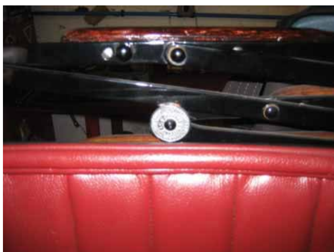
(Left) Maker's cast plate fitted to the hood mechanism. This is a good indicator of an original hood frame, as replica hood frames usually have a flat steel or brass disc. (Right) The wiring beneath the scuttle is largely modern.
