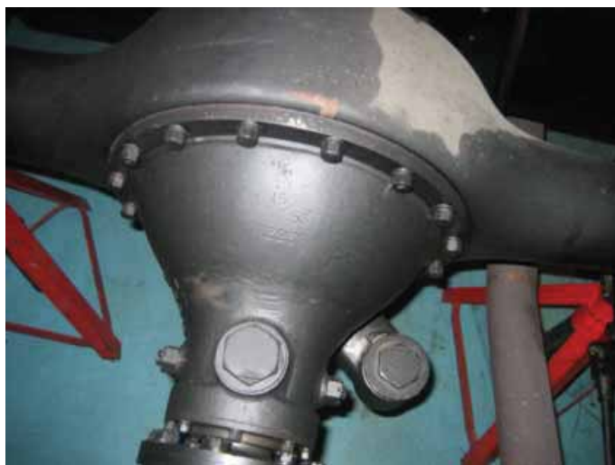
(Left) Back axle banjo and differential casing, both numbered TX3239. The ratio, 15/53, is the standard 3.53:1 ratio for a 4½ Litre. (Right) Nearside rear detail, showing the early pattern B&D friction shock absorbers fitted as standard to the 1928 model 4½ Litre, and standard 4½ Litre tank but with the side filler neck blanked off and extra top filler added (this is a common modification as the original filler neck is a very poor design).
