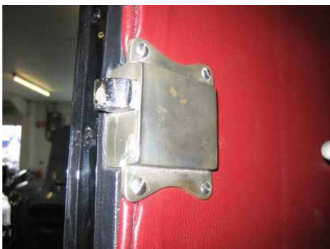
(Left) Original pattern lock as used by Vanden Plas with offset catch (the modern replicas have a central catch). (Right) Original pattern Vanden Plas seat runners, heavy bronze section, with original pattern VdP drop catches engaging in drilled steel plates screwed to the floorboards.
