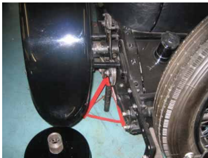
(Left) Back axle banjo and differential casing, both numbered TX3239. The ratio, 15/53, is the standard 3.53:1 ratio for a 4½ Litre. (Right) Nearside rear detail, showing the early pattern B&D friction shock absorbers fitted as standard to the 1928 model 4½ Litre, and standard 4½ Litre tank but with the side filler neck blanked off and extra top filler added (this is a common modification as the original filler neck is a very poor design).
