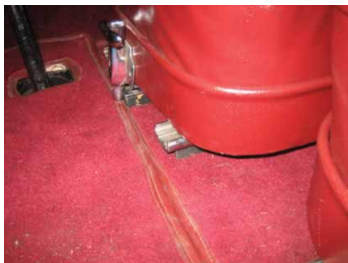
(Left) Original pattern lock as used by Vanden Plas with offset catch (the modern replicas have a central catch). (Right) Original pattern Vanden Plas seat runners, heavy bronze section, with original pattern VdP drop catches engaging in drilled steel plates screwed to the floorboards.
