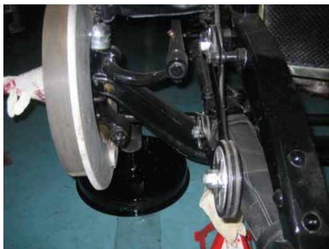
(Left) Detail of front axle beam, stamped TX3239. (Right) Offside front suspension/brake detail. The brakes are the early non-servo pattern, correct for a 1928 model 4½ Litre, as is the early pattern B&D friction shock absorber with long upper arm (the later pattern have a much shorter upper arm).
