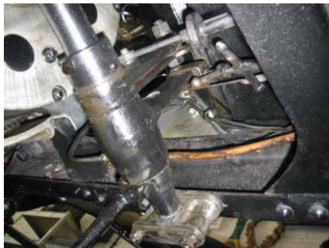
(Left) Detail of the welded-in reinforcing plate to the chassis top flange, nearside, going into the wheel arch. (Right) Detail of the plate clutch with plate clutch pedal shaft fitted by Bentleys in 1931.
