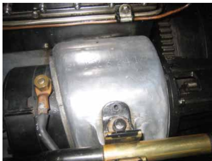
(Left) Nearside of the engine compartment, showing, correct for a 1928 4½ Litre, ML magnetos (either ER4 or GR4), thermostat housing, Smiths starter motor, round flange exhaust manifold, Smiths cut-out and fuse box to the front face of the bulkhead. (Right) Nearside engine bearer showing the original engine number TX3241 and the original pattern clip for the starting handle.
