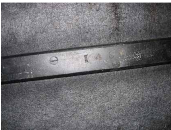
(Above) Vanden Plas body number 1486, stamped into the longitudinal runner to the rear floorboard (left) and the bottom timber to the nearside in front of and to the left of the front passenger seat (right). These numbers were stamped to ensure that floorboards, seats, windscreens, etc went back to the correct bodyshell after going through detail shops at Vanden Plas' works at Kingsbury.
