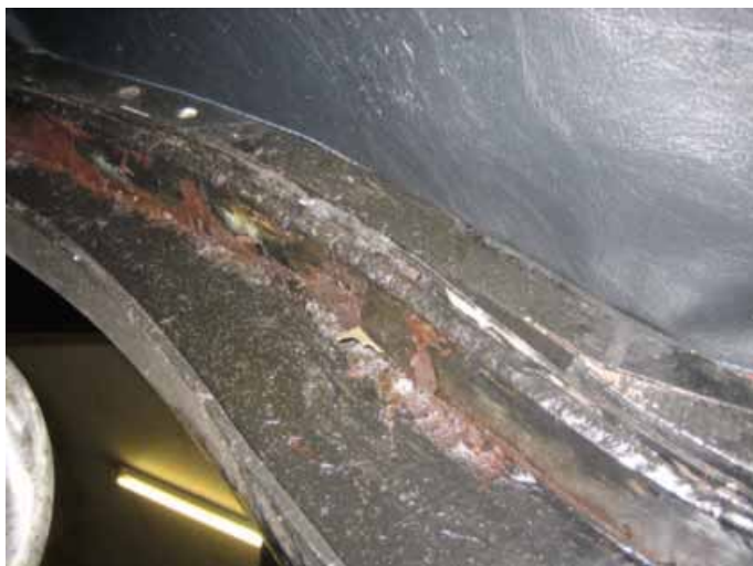
(Left) Detail of the welded-in reinforcing plate to the chassis top flange, nearside, going into the wheel arch. (Right) Detail of the plate clutch with plate clutch pedal shaft fitted by Bentleys in 1931.
