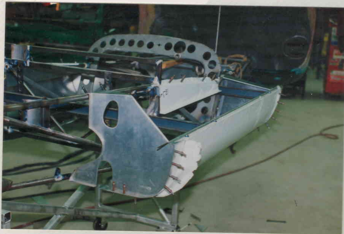
Complete pod assembly tacked in place.
