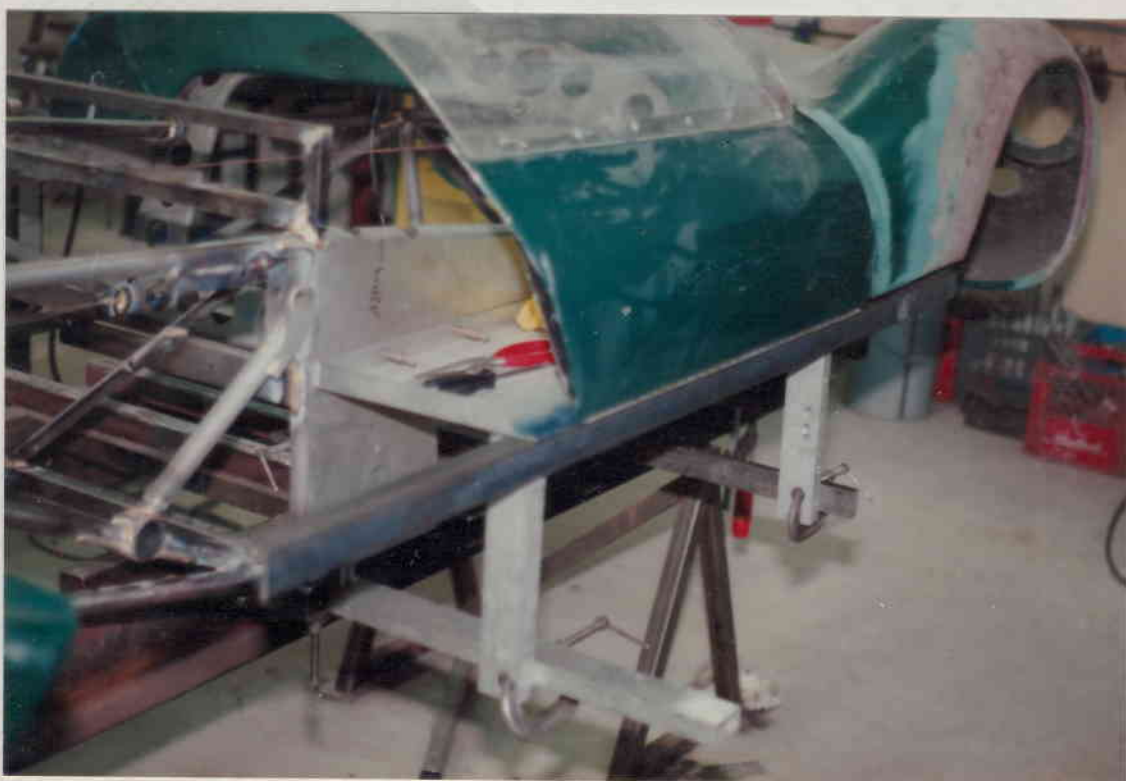
Door mounting to side pod jig.
