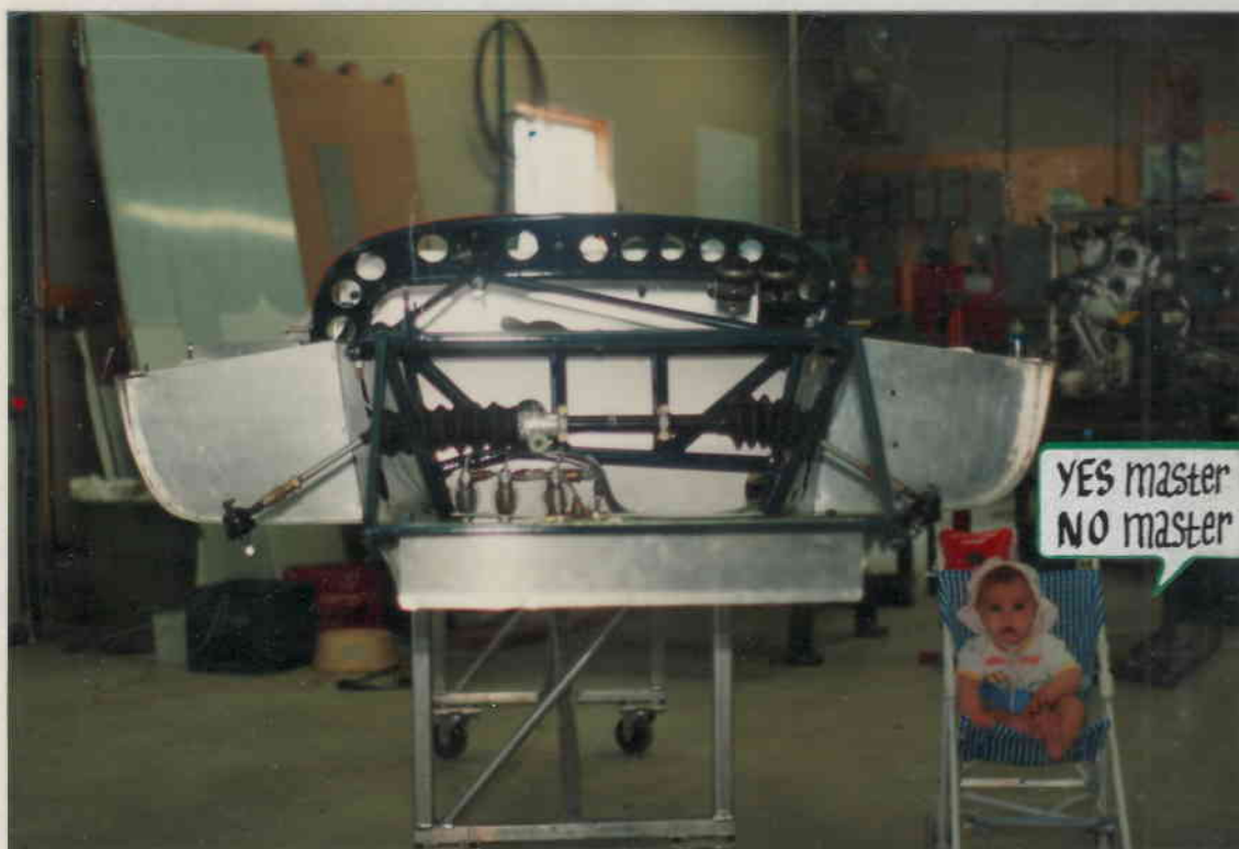
Master cylinders and rack installed...apprentice mechanics are starting younger every year...
