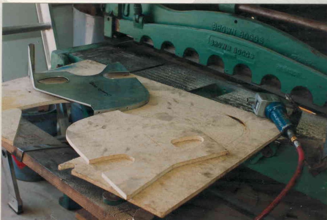
New diaphragm panel showing wood former.
