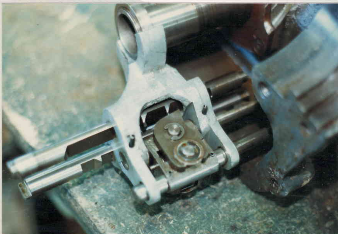
Detail of shifter detent.
