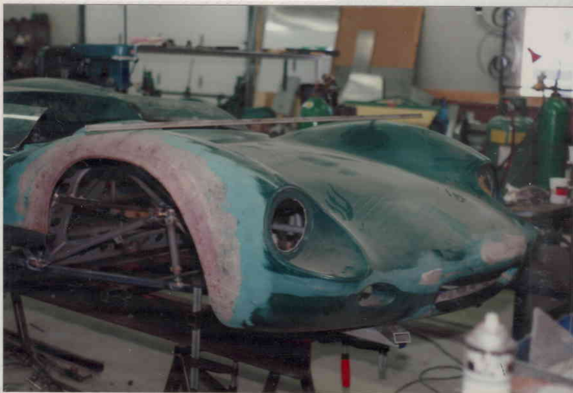
Fitting of nose to frame.
