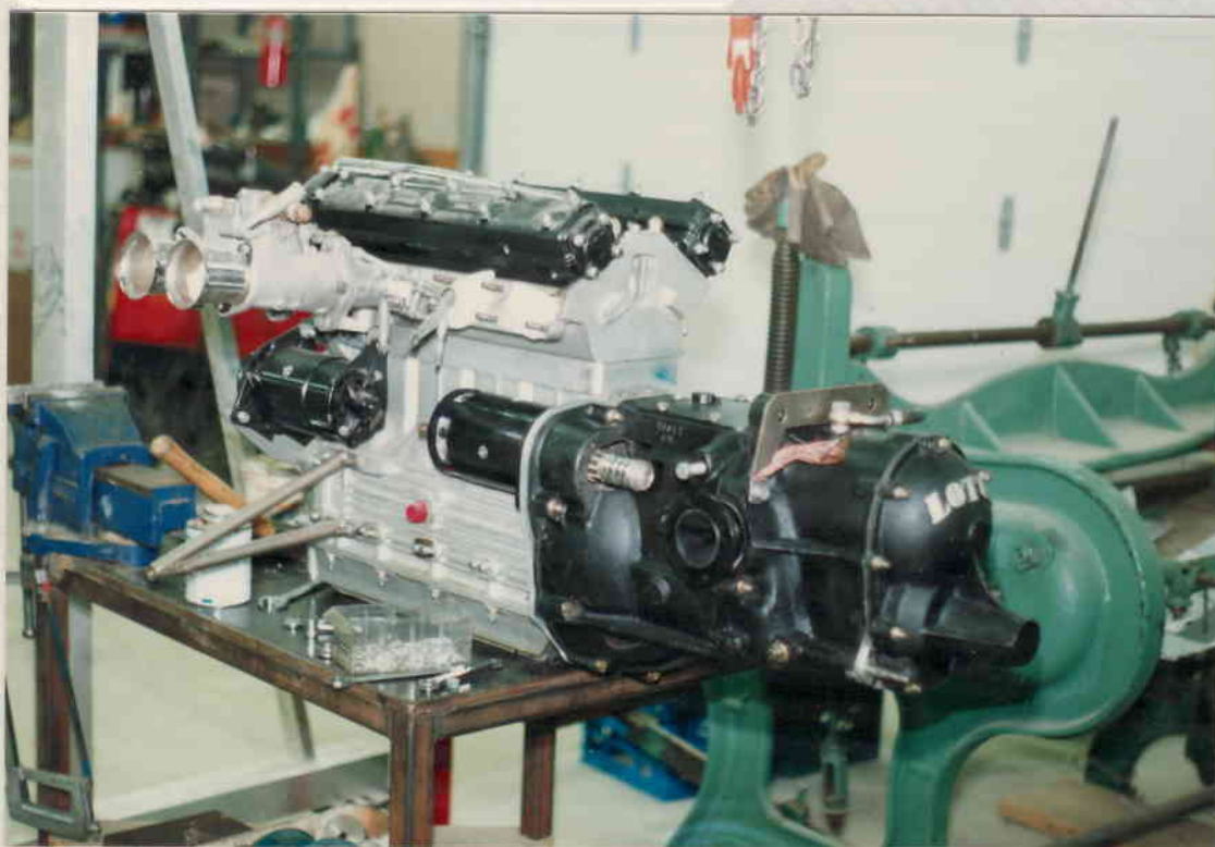
Mounting engine to gearbox.
