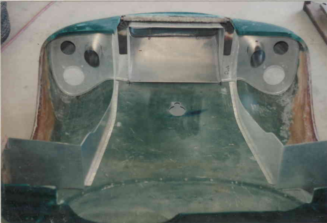
Aluminum inner skins installed in nose.
