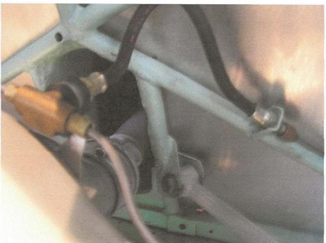
Suspension: Front appears to be completely standard with standard steering arms, except for the aggressive drilling of both the backing plates and brake drums. Rear appears to be somewhat cobbled up with the axle mounting both welded and bolted together, and the curved "A" (panhard) arm is new (this piece required many shims, approx. 5/8" worth, to fit to an Eleven). Rear drums are also drilled for cooling.
